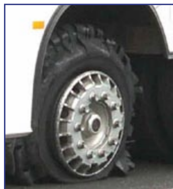
Result of over-inflation of a coach tyre.
