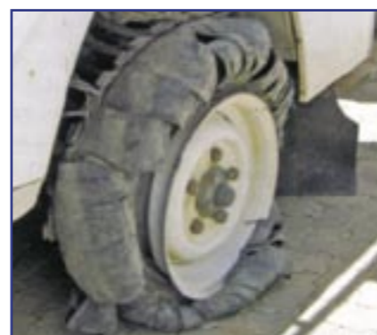
Delamination after driving at 70 mph for fifty miles on a hot road in an ambient temperature of 30°C. The tyre itself was two or three years old with minimal wear, but, it had been used as a spare, riding in strong sunlight on the bonnet of the Land Rover it subsequently caused to be written-off. Please take heed of the advice provided in the article above.
