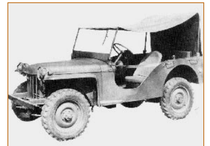
This is the Bantam prototype. It had a proprietary Continental engine that was no match for what Willys had on the stocks and the firm from Butler ultimately lost out. Photo Jim Dunn Collection/US Army.
