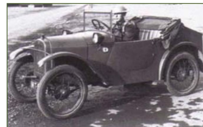
A very early version of the Mulliner Military Seven, probably at Catterick Camp. Note the absence of running boards, shallow door, short bonnet and, of course scuttle-mounted lamps.
