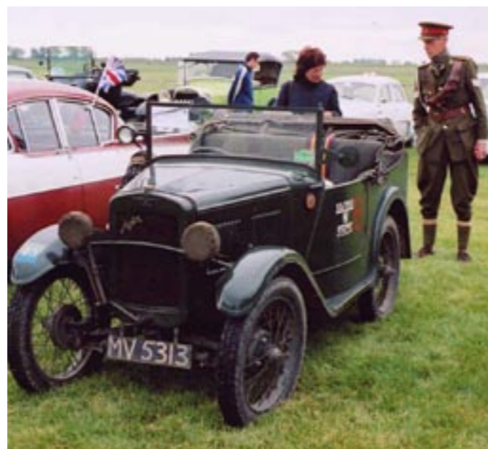
This splendid example of a wireless car is attending a recent rally in Holland with its 'period' owner. The towing rings on the wheel centres can just be seen but the stowage area at the back is clearly visible. The screen mounted spotlight often had a driving mirror on the back and the method of raising the starting handle higher than normal is also interesting Photo PWA7C.
