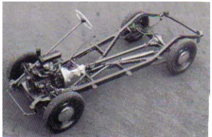
The chassis was a conventional cruciform braced affair but with a new ohv engine that was lively, straightforward, reliable and durable. Photo Austin Motor Co.
