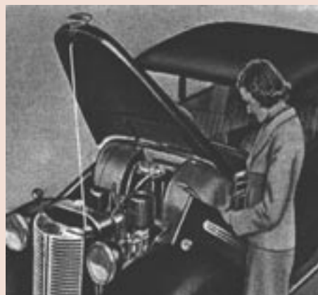
There was a brand new 'alligator' bonnet and detachable side panels to facilitate access to the engine.
